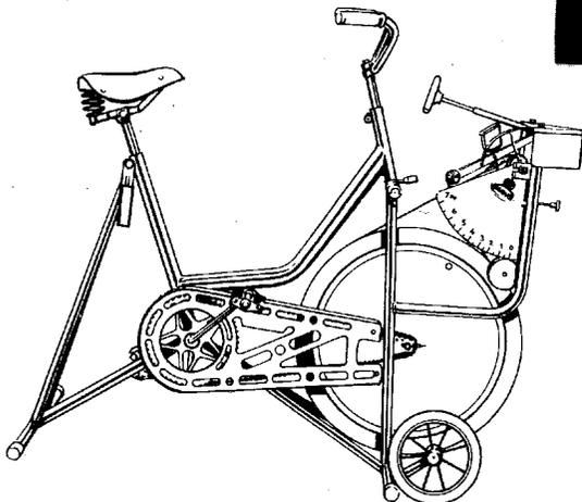
The ergometer cycle is designed for exact measurement of work carried out. This makes it possible to carry out precision determinations of work carried out and follow the condition. Used for scientific purposes, in hospitals, gymnasiums, etc., but also useful in connection with training for those who prefer to have exact control over the degree of loading.
