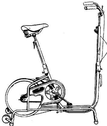
Collapsible exercise cycle. Fitted with small wheels on which it can be put out of the way when not in use.
